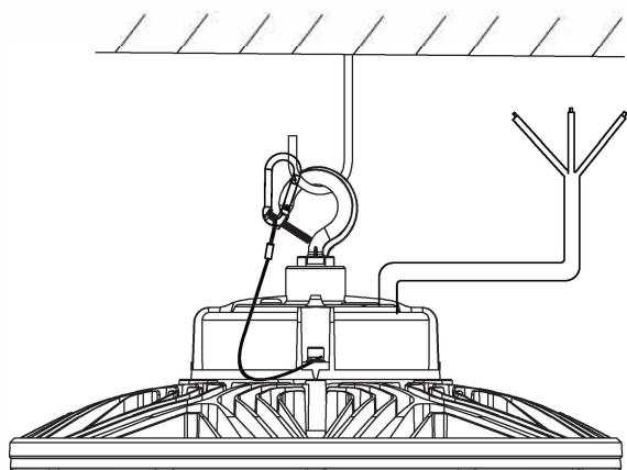
5. Connect wires as below diagram and turn on power to lighting.
