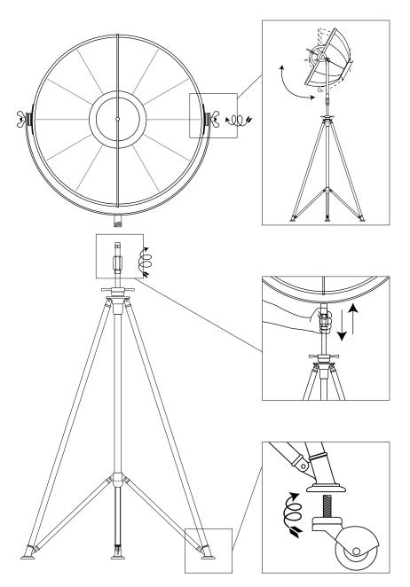
To tilt head, loosen the wing nuts (G), select the prefered position of the head, then tight the wing nuts (G).
